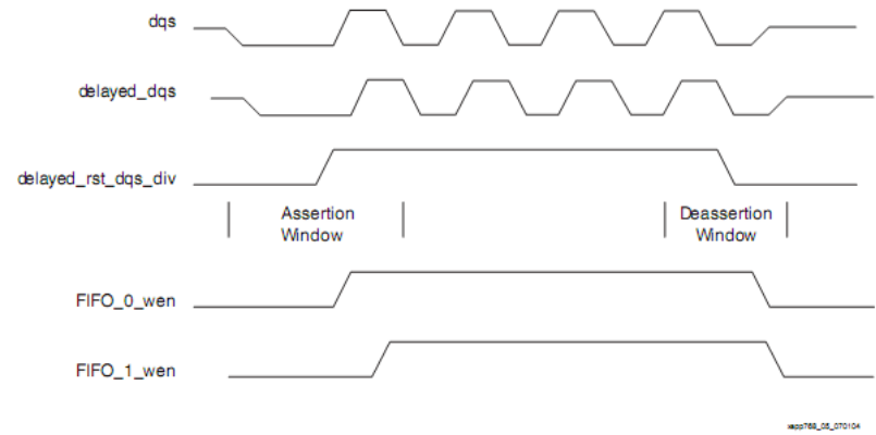
Figure 5: FIFO Write Enable Timing Diagram
